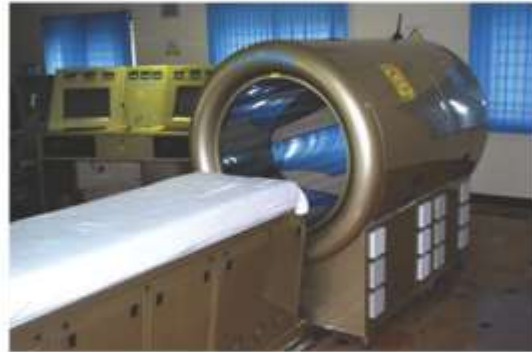
Figure 1A: The CYTOTRON® whole body device. The CYTOTRON-RTE-604D-864GEN (Class IIA Medical Therapeutic Device, developed by Scalene Cybernetics Ltd, Bengaluru, India) is seen in the foreground. The wide-bore gantry houses 864 guns distributed in 9 axes; with each axis bearing 96 guns to deliver RF & MR as per protocol; a moving patient bed and built in device control unit. The central control & command computer for dosimetry planning is seen in the background.
